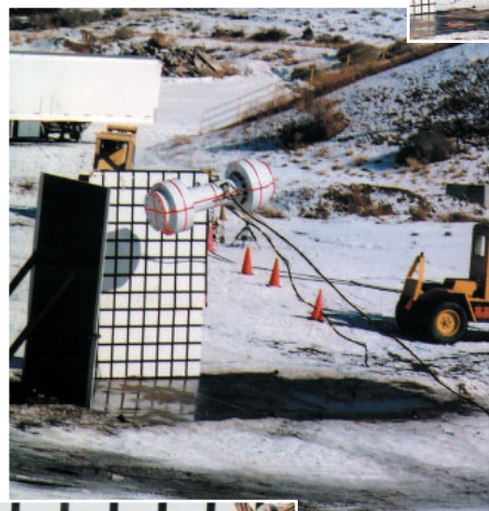
A scale-model container "drop test" helps researchers understand the forces involved in typical and unusual crash situations.
