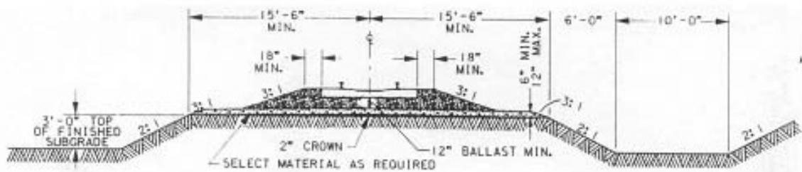
**Figure 21: Typical Railroad Cross-Section**
