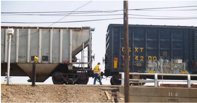
A worker removes the coupling pin between the two cars.
